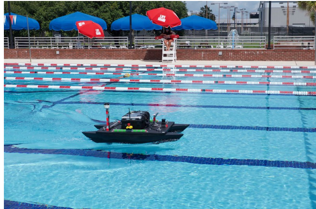
Fig. 6: Ragin' Cajun RoboBoat Performing System ID Trials
